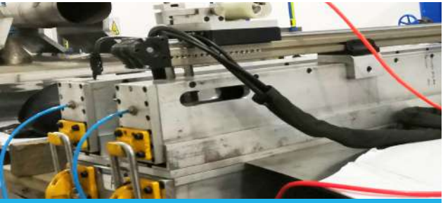
横向焊接 Cross welding
